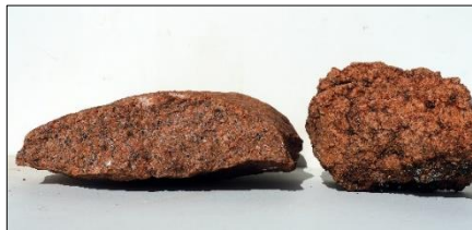
Hiltaba Granite (L) with coarse crystal texture and weathered equivalent (rotted grus) (R)
